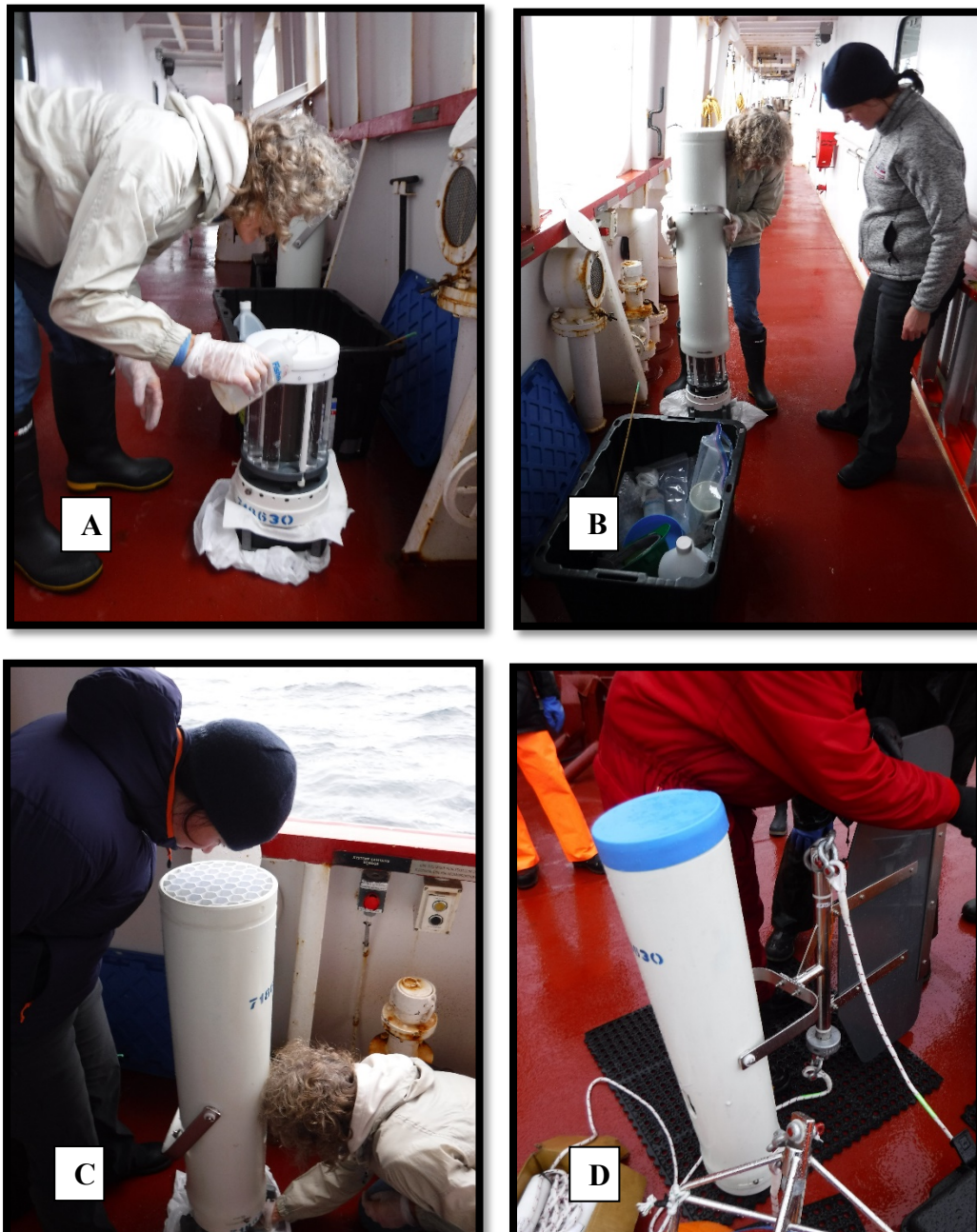
Figure 9. Sediment trap equipment, methods and deployment
